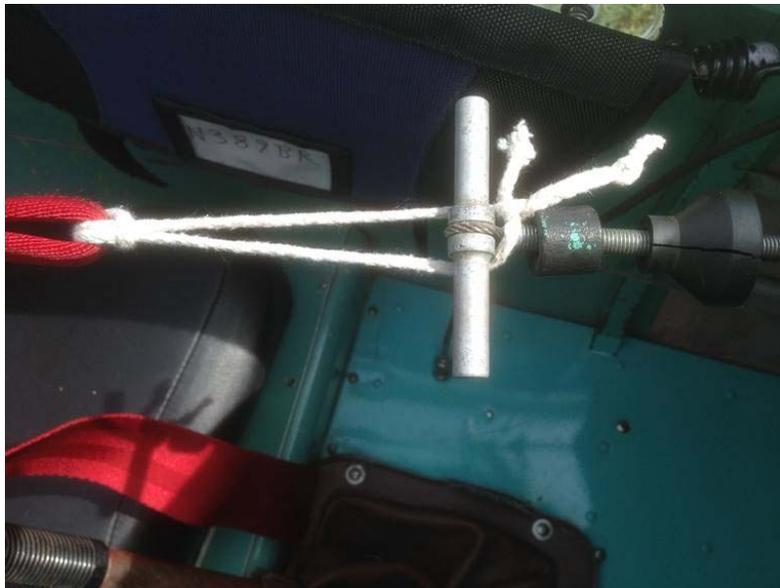
With the strap adjusted close to its shortest possible setting, this will hold the spoilers fully open.
